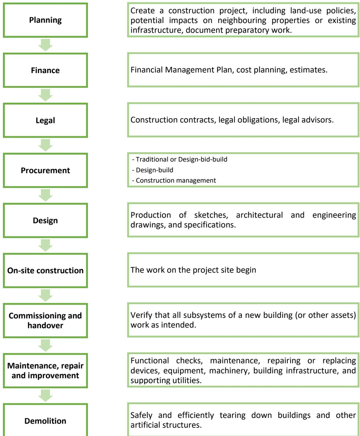
Figure 1. Construction Processes (Source: <https://en.wikipedia.org/wiki/construction>)
